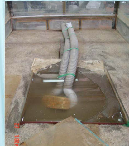
6* 1.5m Flume Open Channel for Reservoir Modeling with Mechanical Sediment Leveler
